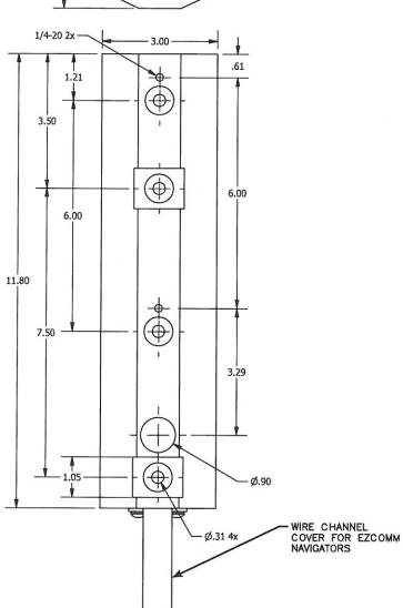
This adapter is designed to mount a Navigator on a non-round decorative or fluted pole. The adapter can either be strapped to the pole or bolted to the pole. Adapter is fully compatible with N2 (Wire Channel Cover not needed) and EZComm Navigators (Wire Channel Cover needed).
